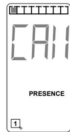
**Step 1:** Observe a single standard automobile in the loop zone. Note the number of segments displayed on the bargraph. **(4)**
